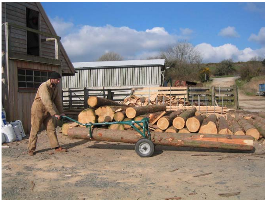
(3) Log is then balanced, up off the ground and on two wheels.
