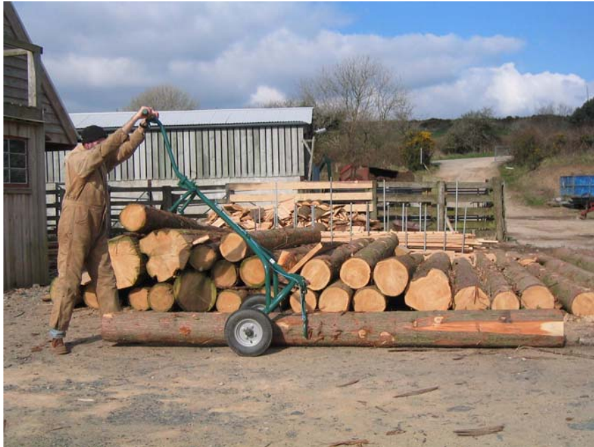
(2) Pull Handle downwards, engaging the tongs and lifting the Log
